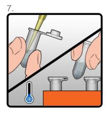
Process the collected sample immediately or store at refrigerated temperatures (depending upon the specific application) until required.
