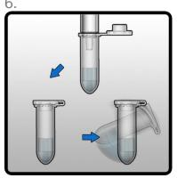
Gently remove the Eppendorf Tube from the end of the Compression Tube. It is appropriate to remove the Eppendorf Tube during expression if necessary due to foaming. Add preservative (not provided), if required, and close the lid on the tube tightly.
