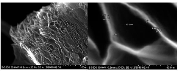
High resolution SEM of rGO powder: Left: The layered structure of rGO is clearly observable for rGO particle. Right: Individual sheets.
