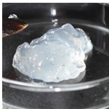
▲(左)Cationically modified CNF, DS=0.0717, concentration;0.93% (右)Un-modified CNF, concentration;1.34%
