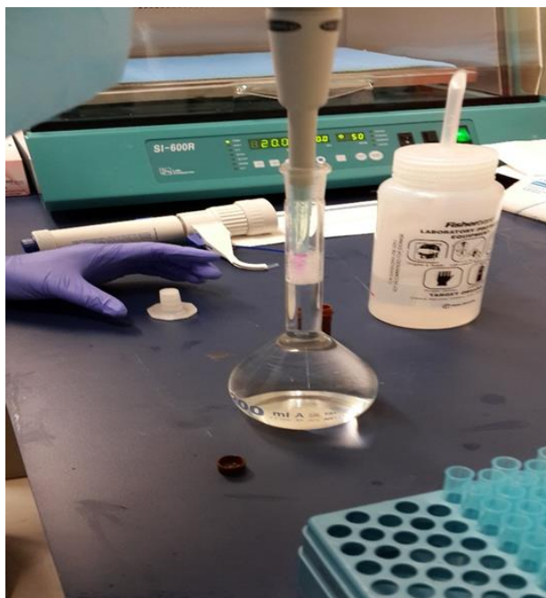
Figure 7: Add 200 \mu l of Cy3 – anti human IgG and 200 \mu l of Cy5-Anti-Human IgA into 200 ml of SAB (1:1000 dilution) in volumetric flask. Invert a few times to mix.
