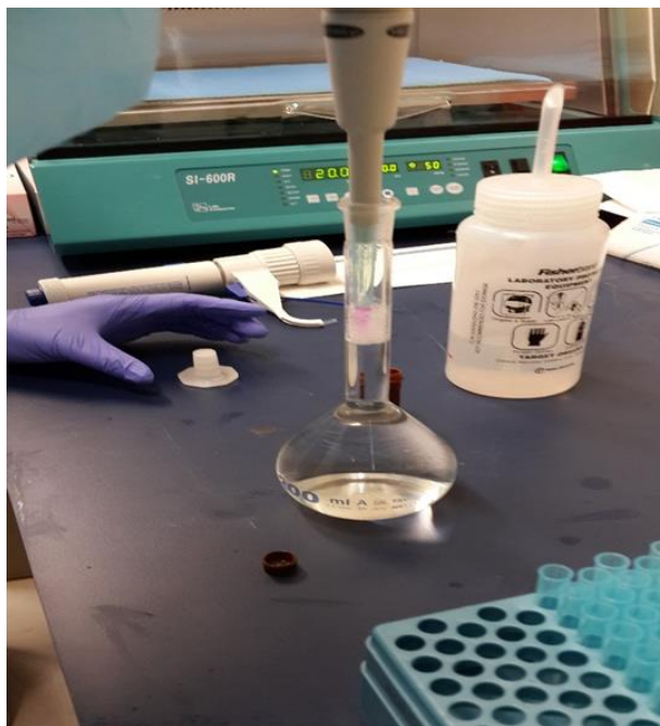
Figure 7: Add 200 \mu l of Cy3 – anti human IgG into 200 ml of SAB (1:1000 dilution) in volumetric flask. Invert a few times to mix.
