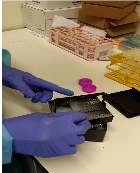
Figure 6: Wash 3; Transfer all slides into slide staining dish with a rack containing 200 ml of SAB.
