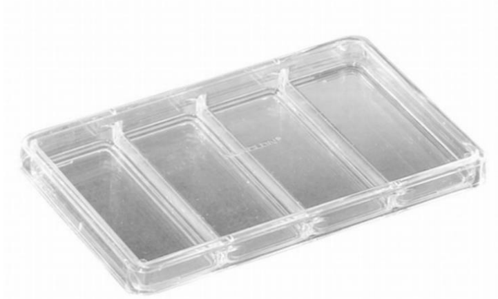
Figure 4. CELLSTAR® FourWell plate dish used for the incubation step of the slides with the sample. The slots in the dish are pre-filled with 4 ml of diluted sample. The slide is gently placed inside the slot. One slide per slot.
