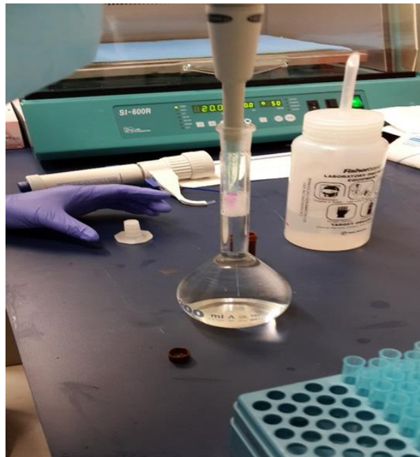
Figure 8. Add 200 \mu l of Cy3 – anti human IgG and 200 \mu l of Cy5-Anti-Human IgA into 200 ml of SAB (1:1000 dilution) in volumetric flask. Invert a few times to mix.
