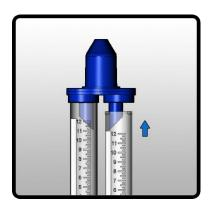
Attach the two Collection Tubes to the bottom of the UltraSal-2™ base by sliding one tube over each outlet and pushing them firmly into the bottom of the base until they snap securely in place.
