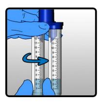
Gently remove the Collection Tubes by holding the UltraSal-2<sup>™</sup> base in one hand, grasping a tube in the second hand, and twisting the tube gently from side to side until the tube separates from the base.
