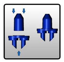
Wearing disposable gloves, snap the mouthpiece securely inside the large ring on top of the base. Label collection tubes as required with sample ID information.
