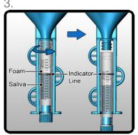
In an upright position, unscrew the Collection Funnel from the Collection Tube by rotating the Collection Tube in the direction shown until the Collection Tube is completely detached from the Collection Funnel.
