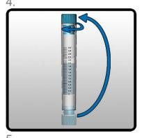
Carefully remove the Tube Cap from the bottom of the Collection Tube and screw the Tube Cap tightly closed on the top of the Collection Tube. Discard the Collection Funnel.
