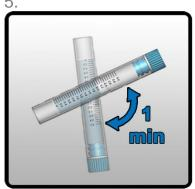
Invert the vial for 1 minute to stabilize the sample.
