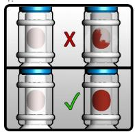
Collect until the appearance of the SVAI changes from white to fully red. The collection procedure should last approximately 1-5 minutes.
