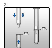
Attach the Eppendorf tube provided to the base of the Compression Tube firmly. Sample collection may now begin.
