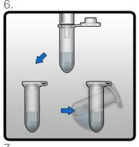
Gently remove the Eppendorf Tube from the end of the Compression Tube. Add preservative (not provided), if required, and close the lid tightly. Invert the tube 2-3 times.
