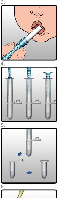
Place the tip end of the white absorbent collection pad of the Micro•SAL<sup>™</sup> device into the mouth of the infant where saliva pools, and collect until the pad is saturated.
