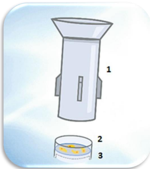
Fig. 2 Part of the filtration set (MetaCell®)—a filtration tube is shown in detail to identify specific parts of the filtration tube used in the protocol description. (1) filtration tube (2) plastic ring—a holder of the separation membrane (3) separation membrane
