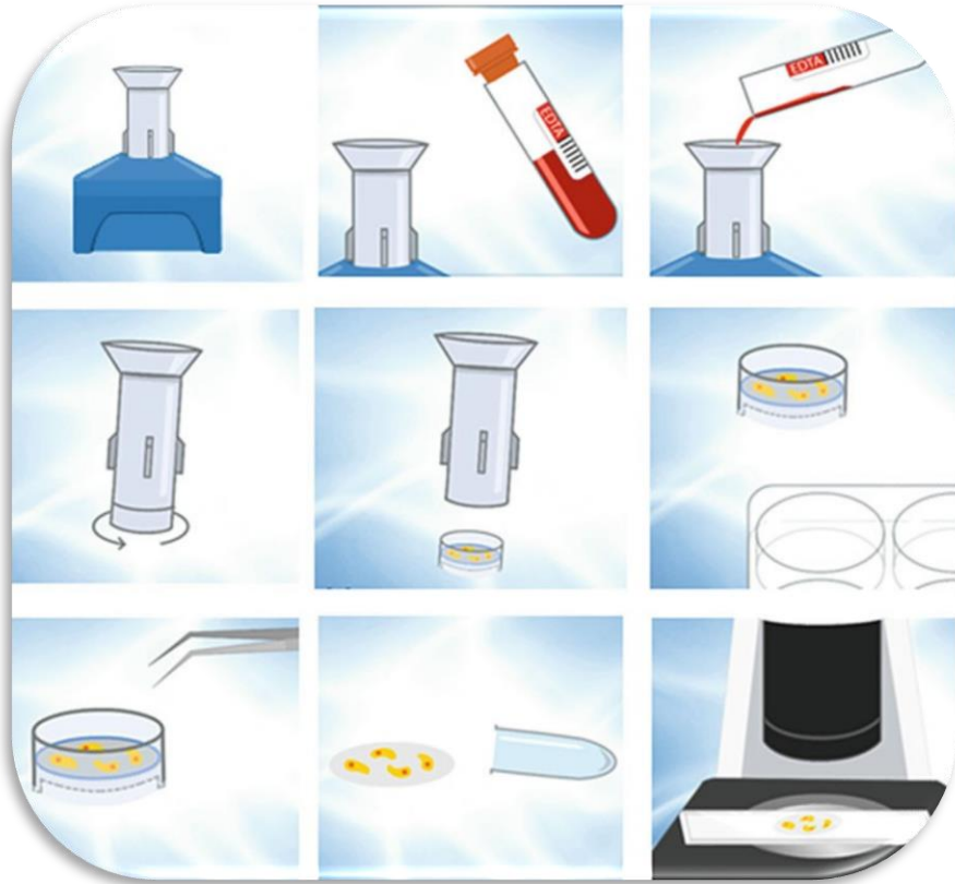
Fig. 1 Filtration procedure as presented by MetaCell is shown in short. Blood is transferred into the separation tube. The filtration starts as soon as the separation membrane touches the absorbent mass placed in the blue separation tube holder. After the filtration process the plastic ring with the separation membrane can be removed and placed directly into the culturing wells. After the short incubation period (min. 72 h) the membrane can be taken out of the plastic ring, the cells on the membrane are cytomorphologically evaluated and/or stored for later RNA/DNA analysis in Eppendorf tubes
